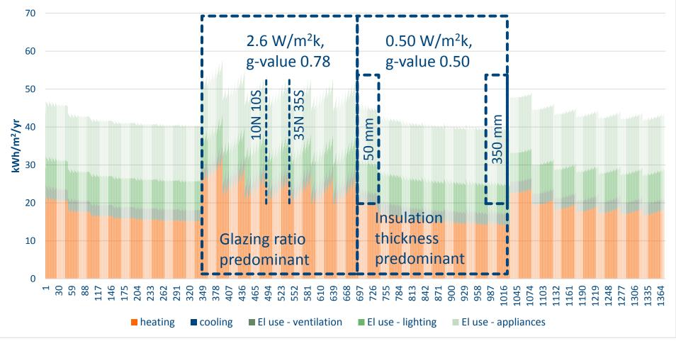
Comparison of results for different combinations of paramenters: operational energy use
