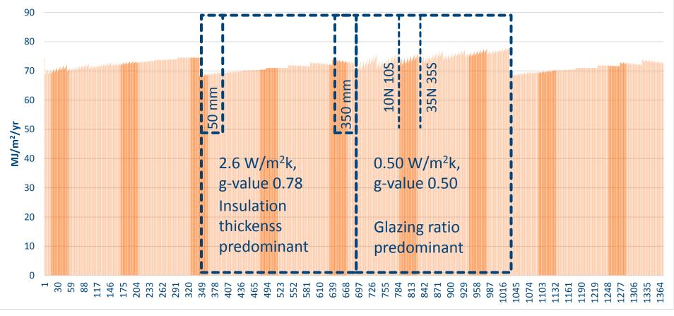
Comparison of results for different combinations of paramenters: embodied energy.
