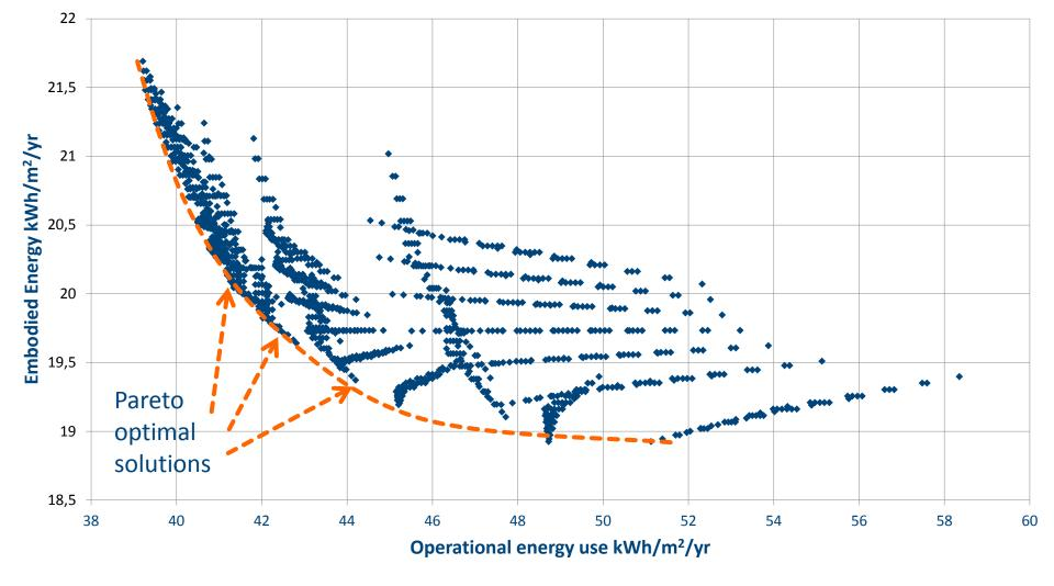
• Comparison of results for different combinations of paramenters: embodied energy vs operational energy use.
