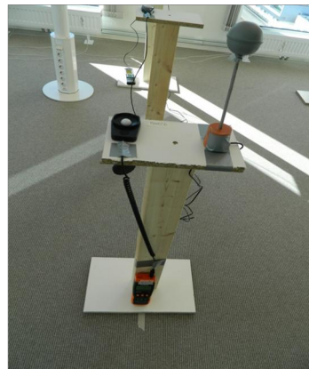
Figure 8: Photo of instrumental setup, illuminance meter (0,85 m) globe thermometer (1,1 m). Photo: Silje Bjørkeng
